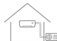
EXEMPLE DE SOLUTION MONOSPLIT AVEC LE MODÈLE ZENKEO
