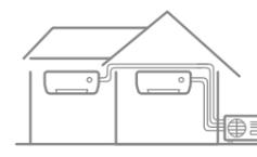
EXEMPLE DE SOLUTION MULTI-SPLITS AVEC LE MODÈLE TAKAO M3 DANS 2 PIÈCES
